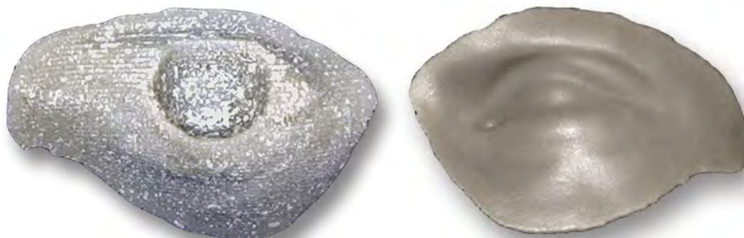
Figure 6a4. The down facing (left) and up facing (right) of the ThermoJet pattern
