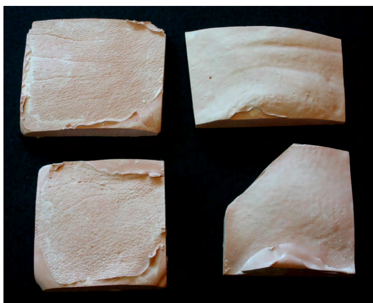
Figure 6b12. Casts produced directly from impression (left) and from impressions of the computer data which were fabricated using ThermoJet (right)
