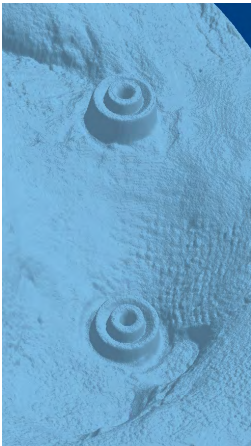
Figure 6g1. Abutments captured by a Roland Picza touch probe scanner (0.05mm point spacing). The data has undergone a smoothing operation. This data represents the benchmark in quality and detail due to the high resolution and lack of noise.
