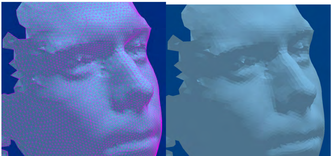
Figure 6g7. The results of a scan using a 3DMD DSP400. The resolution is much lower than the other scanning technologies noted and has resulted in larger triangles. Details around the eyes and nose have been lost.
