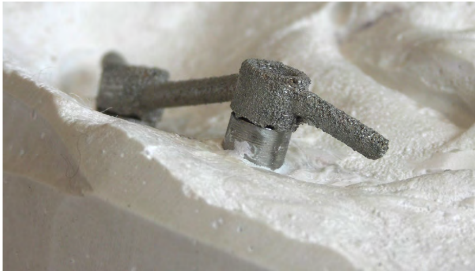
Figure 6e9. SLM bar fit (before polishing)
