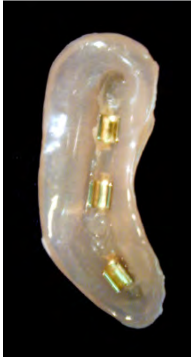
Figure 2.10. A sub-structure shell, incorporating gold clips.
