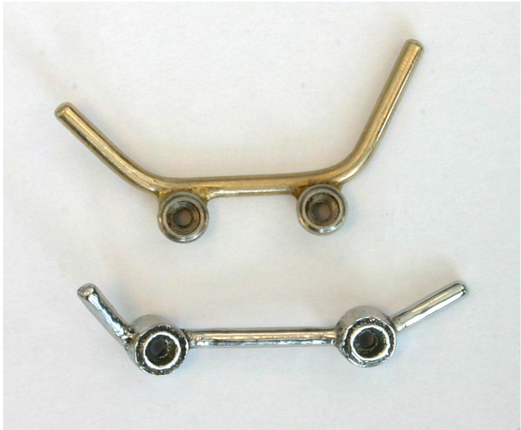
Figure 6e8. A conventionally produced bar (top) and the SLM bar (bottom)
