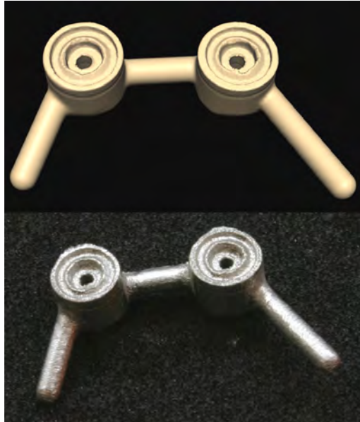
Figure 6e4. The fitting surface of the bar in CAD (top) and SLM bar (bottom)
