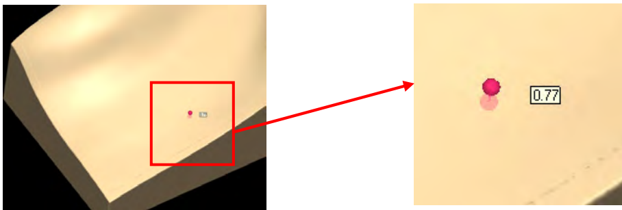
Figure 6b8. Verifying wrinkle depths using the ruler tool in FreeForm
