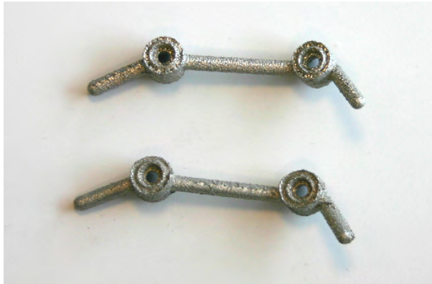
Figure 6e6. Comparison of the fitting surfaces with the bar built with the top surface facing down (top) and standing vertically (bottom).
