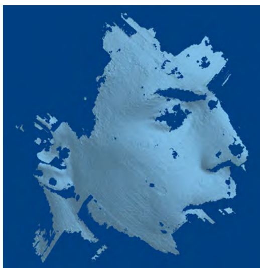
Figure 3.3. Holes in scan data due to reflective surfaces, hair and areas hidden from the line of sight. Data from the Handyscan 3D.
