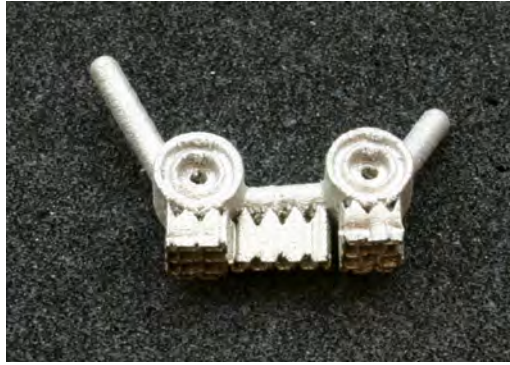
Figure 6e3. The SLM bar with support structure still attached.
