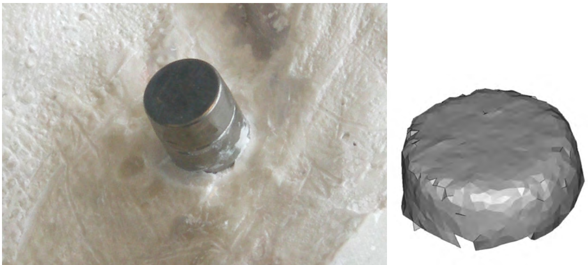
Figure 3.4a (left). A magnetic keeper. Figure 3.4b (right). A scanned magnetic keeper converted to an STL file.
